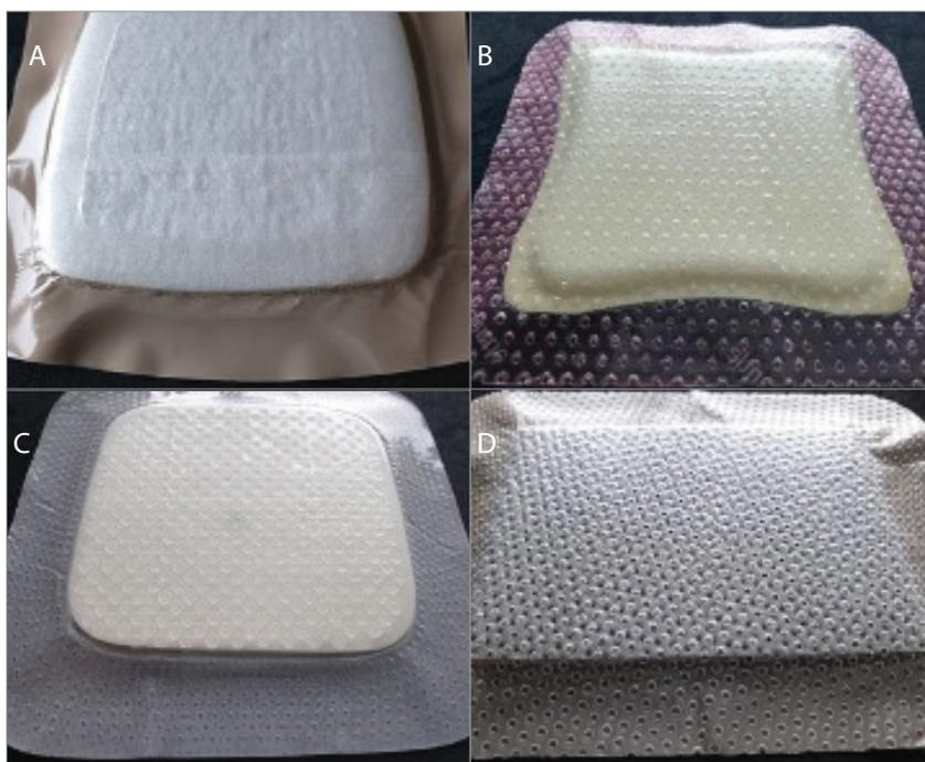
the foam and discarding it, accurately cutting a 2x2 cm sample of the remaining dressing ( $n=3$ ), adding 10 mL of 12.8M nitric acid, subjecting this to closed-vessel microwave-digestion (CEM MARS6) for 20 minutes at 210°C, neutralising with 25 mL of concentrated ammonia solution, diluting volumetrically to 500 mL with deionised water and finally, and filtering through a 0.45 µm
